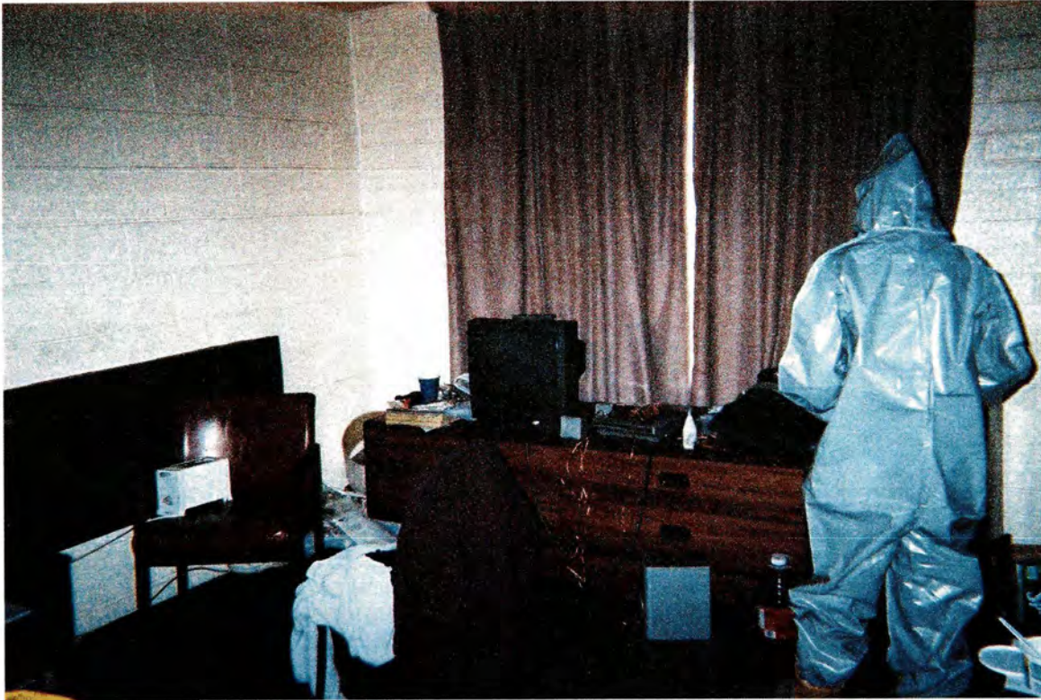
PHOTO 3 START2 monitoring room 111 for mercury vapors.
