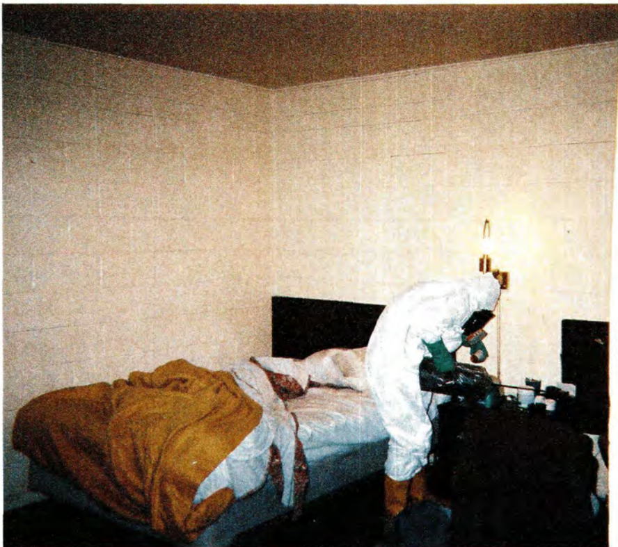
PHOTO 2 START2 monitoring Room 111 for mercury vapors.
